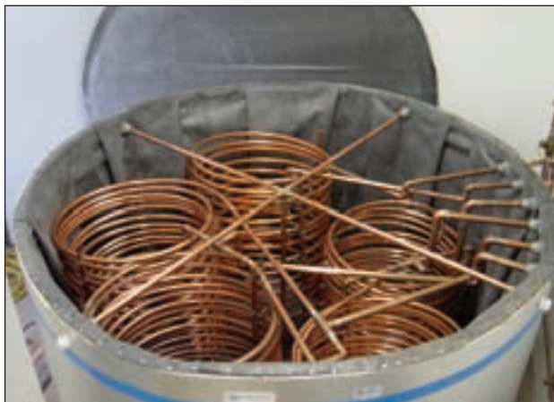
EPDM lined atmospheric drainback tank with copper heat exchanger coils
